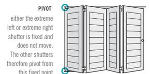
**PIVOT** either the extreme left or extreme right shutter is fixed and does not move. The other shutters therefore pivot from this fixed point
